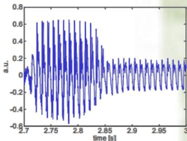
Figure 2. A short segment of speech signal, that may form the input to a hearing aid. The segment displayed corresponds to the sound 'funf'.
