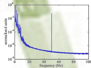
Figure 9. The power spectrum of this signal shows that most of the power is concentrated in frequencies below approximately 20 Hz, with peaks at the heart-rate (about 1.4 Hz) and multiples of this frequency (the harmonics). In addition there is a sharp peak at mains frequency (50Hz).
