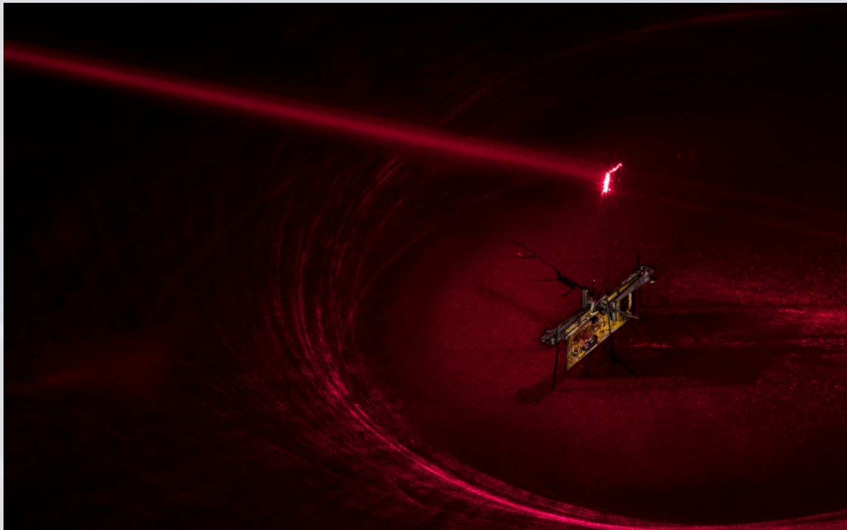
Fig 2 Laser light bathes a photovoltaic cell, providing RoboFly with the power to take flight.
